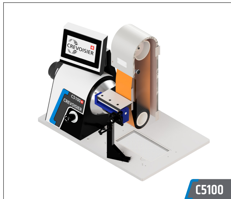
C5100 machine in vertical satin-finishing configuration See the specific chapter for the accessories
