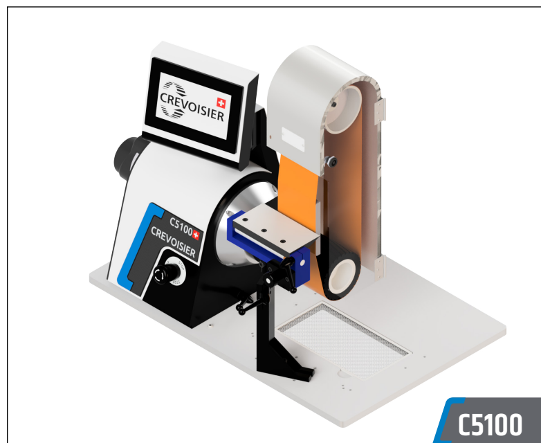
C5100 machine in vertical satin-finishing configuration
