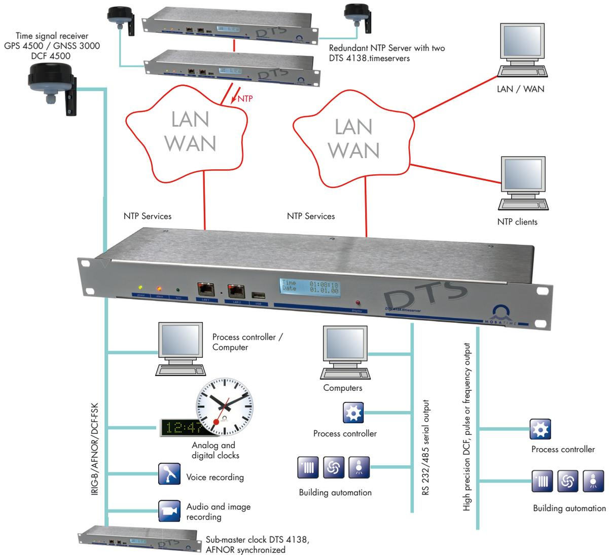
DTS 4138.timeserver features one IRIG-B/AFNOR output to synchronize analog and digital slave clocks, process controllers, voice recording systems and many other technical equipment.
